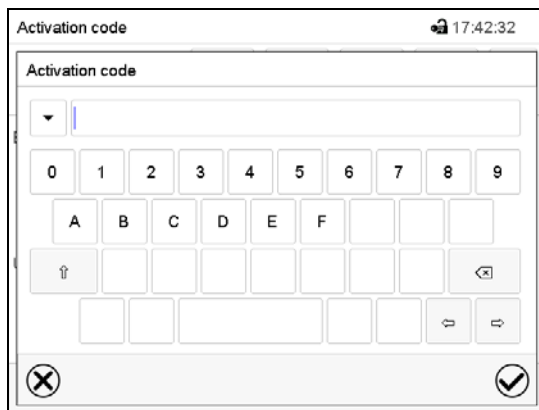
Activation code entry window. Enter the first four characters of the activation code and press the Confirm icon.
