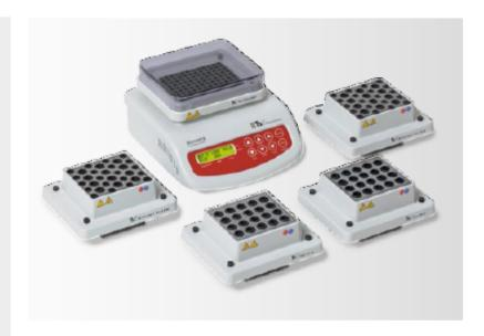
The Biometra TSC ThermoShaker is a thermomixer with heating and cooling function, as well with a variable mixing speed from 250 rpm to 1,800 rpm. Active cooling with Peltier technology allows a temperature adjustment from + 4 °C to + 100 °C.
