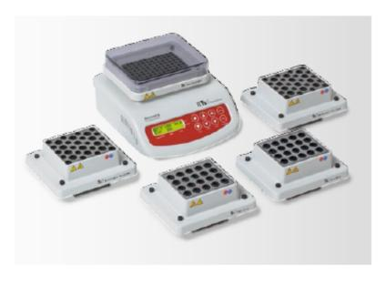
The Biometra TSC ThermoShaker is a thermomixer with heating and cooling function, as well with a variable mixing speed from 250 rpm to 1,800 rpm. Active cooling with Peltier technology allows a temperature adjustment from + 4 °C to + 100 °C.
