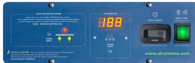
FSA/Autocal Control Panel
