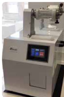
Figure 3: Random Access Sealing Procedure using the a4S RA Automatic Random Access Heat Sealer (4ti-0675, prototype shown)
