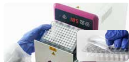
Figure 2: Random Access Sealing Procedure using the 4s3™ Semi-Automatic Sheet Heat Sealer (4ti-0655)
