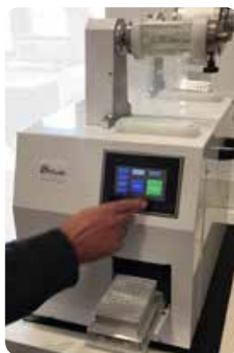
Figure 3: Random Access Sealing Procedure using the a4S RA Automatic Random Access Heat Sealer (4ti-0675, prototype shown)
