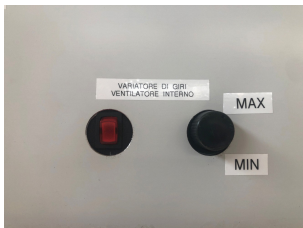
Internal ventilation fan speed variator (optional)
