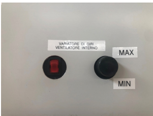
Internal ventilation fan speed variator (optional)
