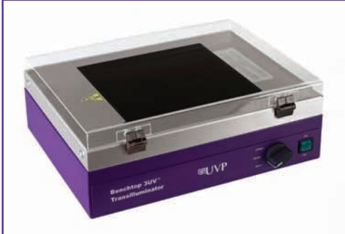
Unique 3UV benchtop models allow researchers to switch between 254, 302 or 365nm UV wavelengths in one unit.
