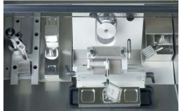
Cryoembedding components in the Leica CM1850 cryochamber
