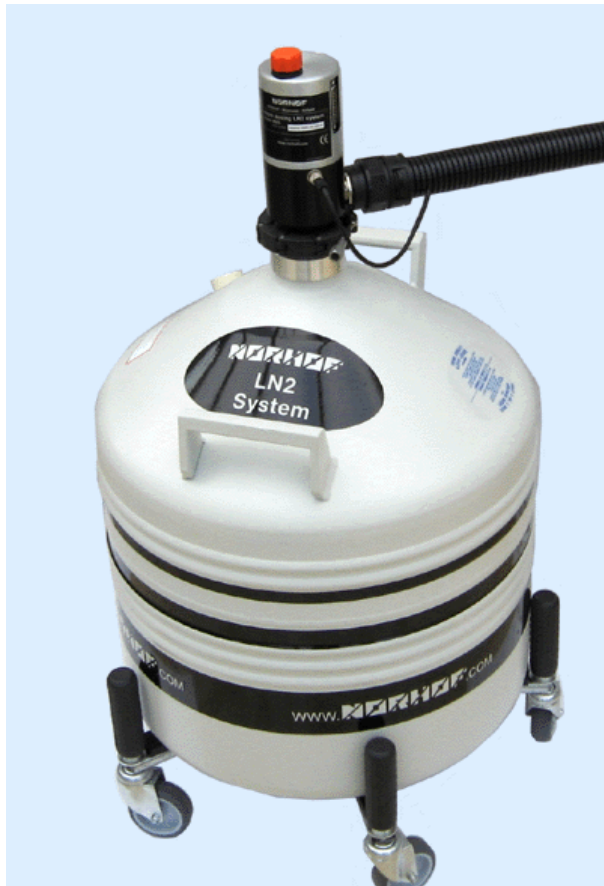
picture shows pump mounted on a 35 Liter dewar, total system height 79 cm
