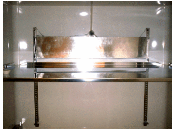
Cold exchanger inside freezer, in the top
