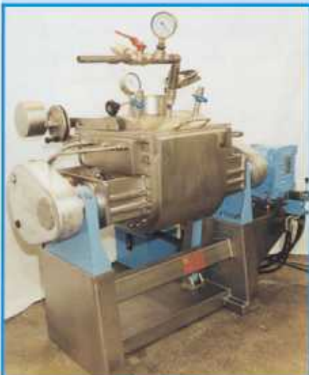
Model MZ35 with high temperature oil jacket (300°C), heavy duty 4kW flameproof drive, mechanical seals and vacuum lid
