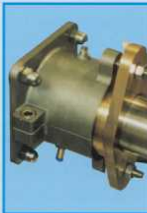
Fully adjustable packing glands showing ample space for adjustment. The split and removable housing (fitted on models MZ35 and MZ75) allows faster cleaning and maintenance of the seals.
