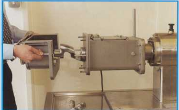
Easy to clean: The trough, blades and drive endplate can all be removed in less than one minute
