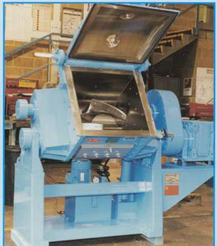
Model MZ75 with stainless steel replaceable liners in trough and replaceable wear strips on the 'Z' blades. Jacketed for high pressure fluid circulation and with hinged, domed lid
