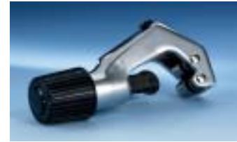
TC2 Heavy Duty Tube Cutter • For clean cuts in hard or soft copper aluminum, brass, thin wall steel and stainless steel. • Rollers have flared cut off groove • Complete with foldaway reamer blade and spare cutting wheel. • Cuts tubes from 1/8" thru 1 1/8" O.D. • Replacement cutting wheel p/n TC2W
