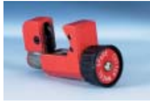
TC1 Mini-size Tube Cutter Easily cuts tubes from 1/8" thru 5/8" O.D. capacity. Requires only 1 5/16" clearance space. (Replacement cutting wheels available: Part No. TC1W)
