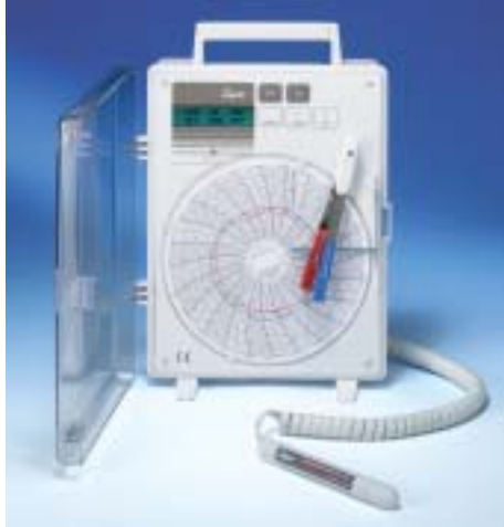
CR4 & KTH (CRTH2) Universal Recorder with Temperature Humidity Probe
