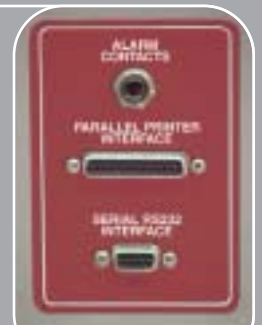
outputs to data logger
