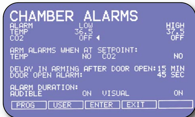
Chamber alarm screen enables password protected alarm setting and easy access to any alarm information.
