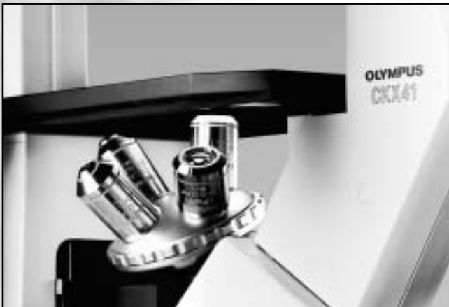
New UIS objectives give better contrast, resolution and working distances.
