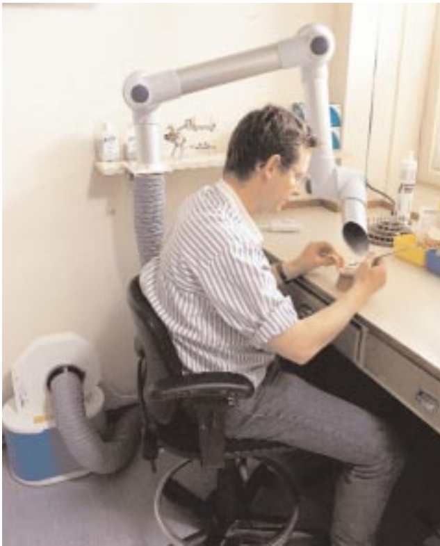
The arm is quickly mounted with the flexible bench bracket and within a couple of minutes the Kit is ready for use.
