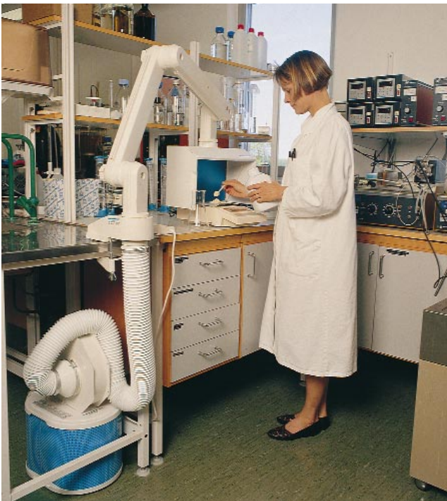
The flexibility of the arm and the different set up of the hood creates a workplace with efficient extraction of fumes and gases.
