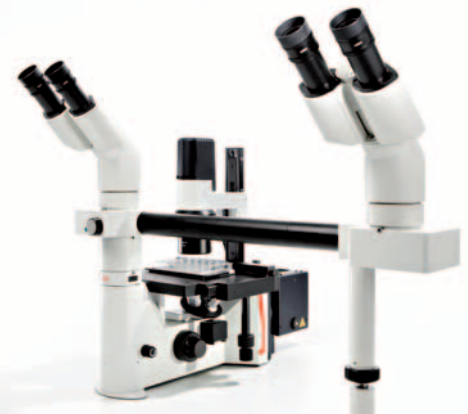
Discussion attachment for two observers on the Leica DM IL LED
