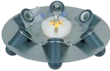
Disc rotor, 6-place, for Schlenk tubes, n = 2,000 \text{ min}^{-1} , RCF 805, max. 6 x 50 ml.
