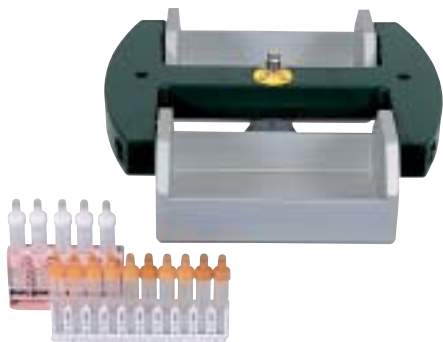
Swing-out rotor, 2-place, for plates and racks, n = 3,600 \text{ min}^{-1} , RCF 2,695, max. 20 racks.
