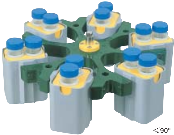
Swing-out rotor, 6-place, n = 4,900 \text{ min}^{-1} , RCF 5,503, max. 6 x 100 ml, illustrated with buckets No. 4396.
