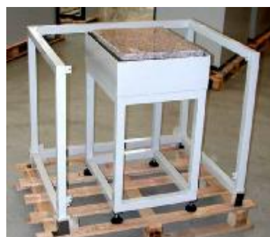
The "double" base-stand support system
