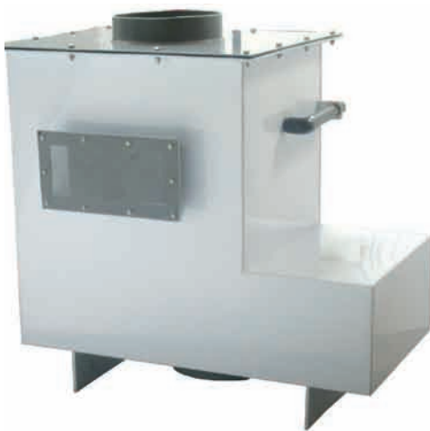
Image 1: Top section of scrubber placed on top of the fume hood. There is an acrylic viewing panel, a packed bed, a liquid spray section as well as a demister in this unit.
