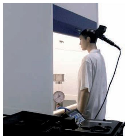
Tracer Gas Containment Test
