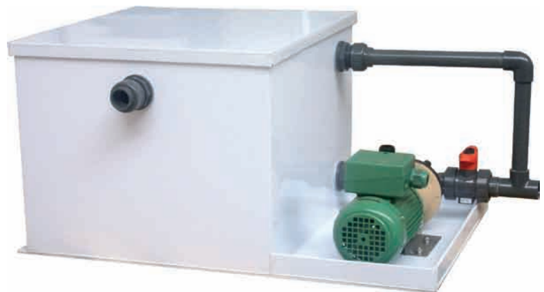
Image 2: Bottom section of scrubber placed inside the base cabinet. Consists of a reservoir for scrubbing liquor and a pump which recirculates the liquor back into the system.
