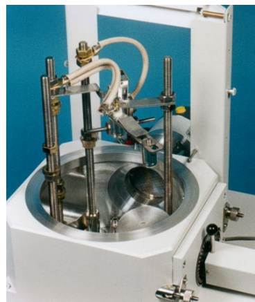
Fig. 12. Multi-source chamber and jigging.
