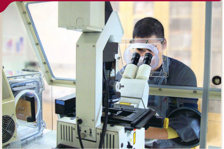
Imaging Glove Box: This alternative to microscope stage chambers and enclosures for live cell imaging provides a constant environment during media change and imaging.
