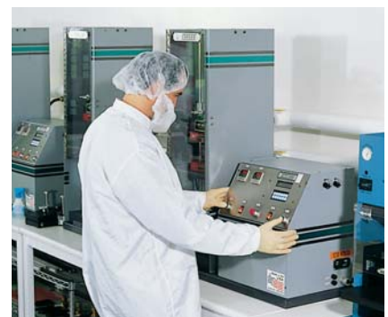
Carver Auto "C" presses molding medical components.*
