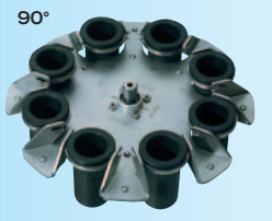
Swing-out rotor, 8-place, n = 4,000 min -1 , RCF 2,415, for 8 x 15 ml, stainless steel, with suspensions No. 01644, PA, fibreglass reinforced.
