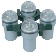
Swing-out rotor, 4-place, n= 4,000 min -1 , RCF 2,665, for max. 4 x 100 ml.
