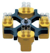
Swing-out rotor, 4-place, n= 4,000 min -1 , RCF 2,665, for max. 4 x 100 ml.
