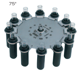
Swing-out rotor, 12-place, n = 5,000 min -1 , RCF 4,187, for 12 x 15 ml, stainless steel, with suspensions No. 01621, PA, fibreglass reinforced.
