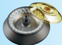
Angle rotor, Cat. No. 01420 24-place, n= 15,000 min -1 , max RCF 21,382
