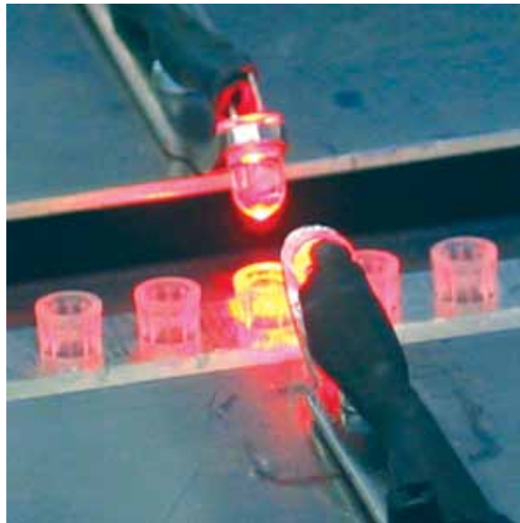
The automatic camera checks each 10 µl Biohit pipette tip thus ensuring the quality control of every individual tip.
